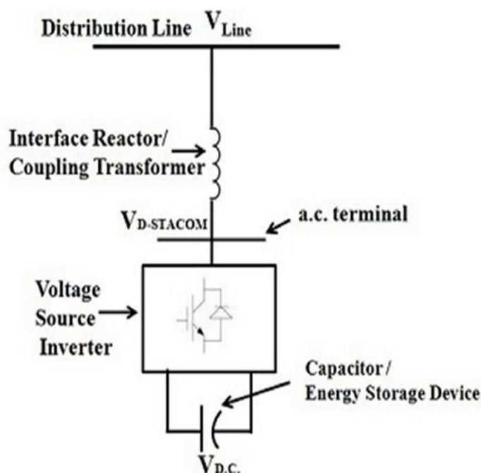
Figure 1: BASIC PRINCIPAL OF D-STATCOM
